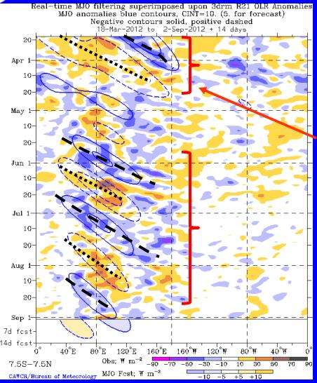
Drier-than-normal conditions, positive OLR anomalies (yellow/red shading)
