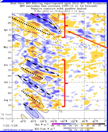
Drier-than-normal conditions, positive OLR anomalies (yellow/red shading)
