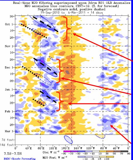
Drier-than-normal conditions, positive OLR anomalies (yellow/red shading)
