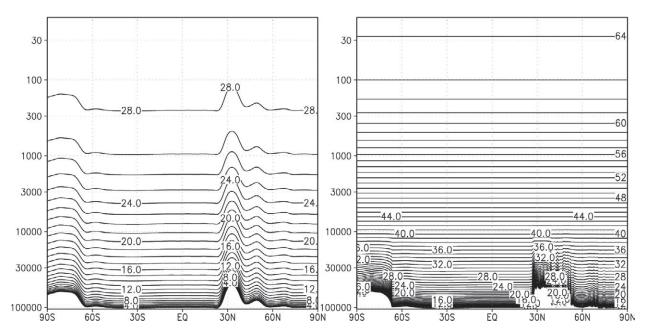
Fig. 10. The vertical structure of model levels as a meridional cross section at 90°E. (left) RI (28 sigma layers) and (right) CFSR (64 sigma-pressure hybrid layers). (top) A linear function of pressure to emphasize resolution in the troposphere; (bottom) log(pressure) is plotted to emphasize stratosphere.
