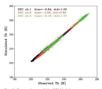
Fig. 6. Comparisons of the SSU brightness temperature at channel I (black), channel 2 (red), and channel 3 (green) between calculations and measurements for Nov 2004.
