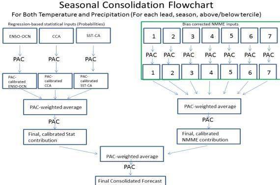
Seasonal consolidation flowchart. The green box indicates process that currently executes operationally upstream of the consolidation. All other processes are included as part of this experimental consolidation process.
