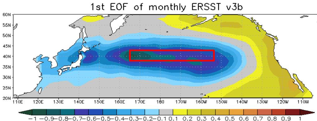
**- Pacific Decadal Oscillation is defined as the 1<sup>st</sup> EOF of monthly ERSST v3b in the North Pacific for the period 1900-1993. PDO index is the standardized projection of the monthly SST anomalies onto the 1st EOF pattern.**
