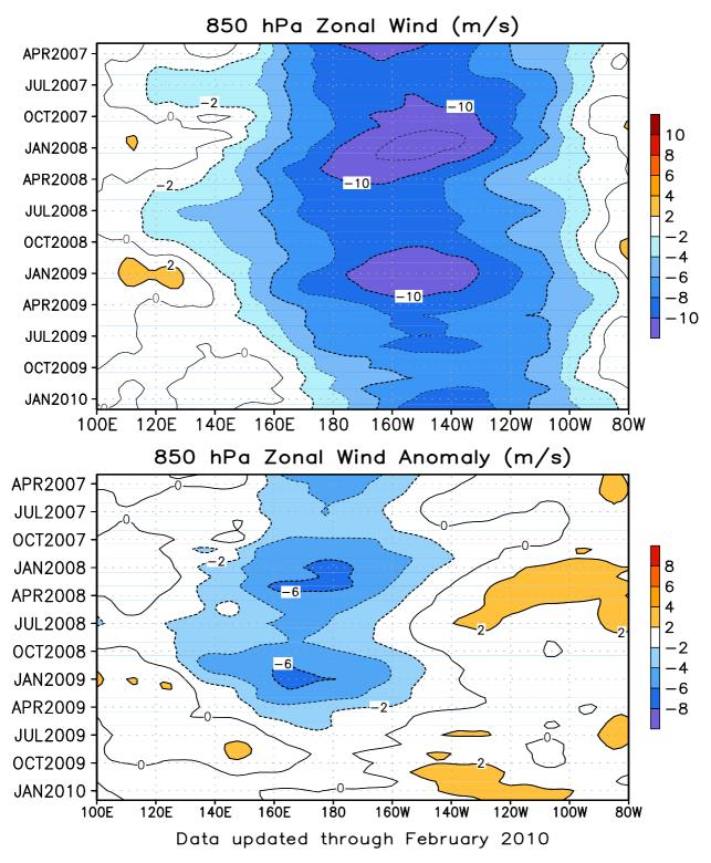
FIGURE T7. Time-longitude section of mean (top) and anomalous (bottom) 850-hPa zonal wind averaged between 5N-5S (CDAS/Reanalysis). Contour interval is 2 ms<sup>-1</sup>. Blue shading and dashed contours indicate easterlies (top) and easterly anomalies (bottom). Anomalies are departures from the 1979-1995 base period monthly means. The data are smoothed temporally using a 3-month running average.
