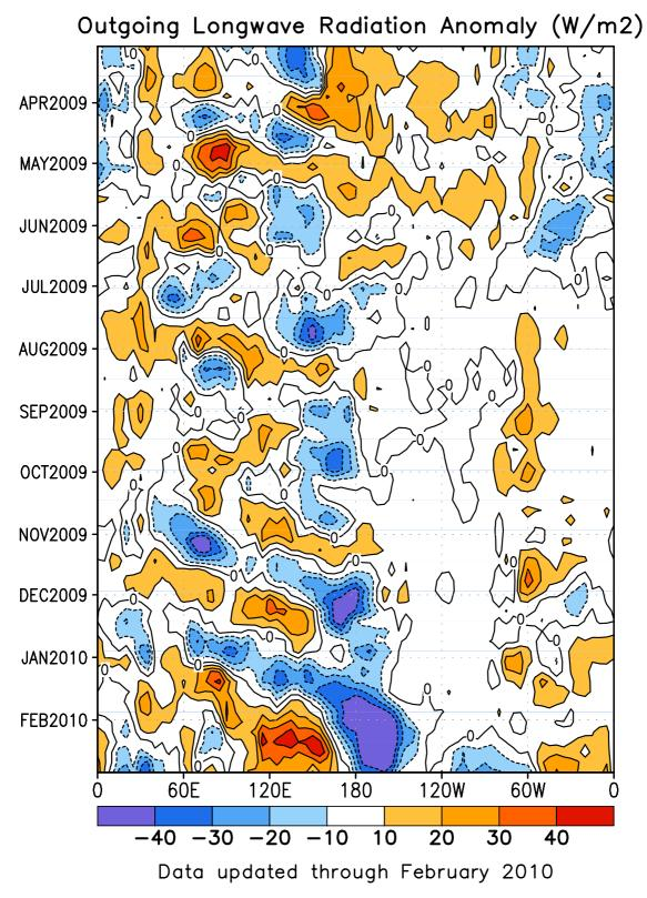
FIGURE T11. Time-longitude section of anomalous outgoing longwave radiation averaged between 5N-5S. Contour interval is 15 Wm<sup>-2</sup>. Dashed contours indicate negative anomalies. Anomalies are departures from the 1979-1995 base period pentad means. The data are smoothed temporally using a 3-point running average.
