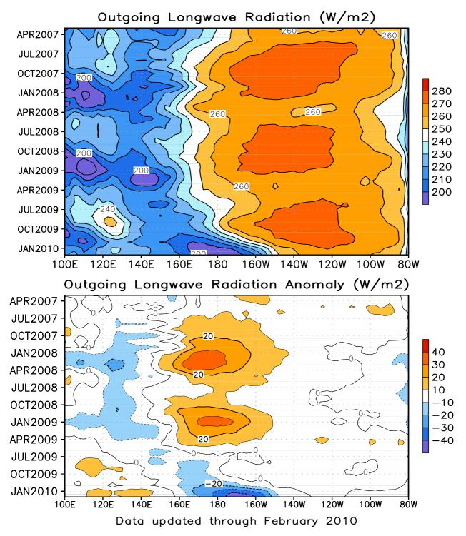
FIGURE T8. Time-longitude section of mean (top) and anomalous (bottom) outgoing longwave radiation (OLR) averaged between 5N-5S. Contour interval is 10 Wm<sup>-2</sup>. Dashed contours in bottom panel indicate negative OLR anomalies. Anomalies are departures from the 1979-1995 base period monthly means. The data are smoothed temporally using a 3-month running average.
