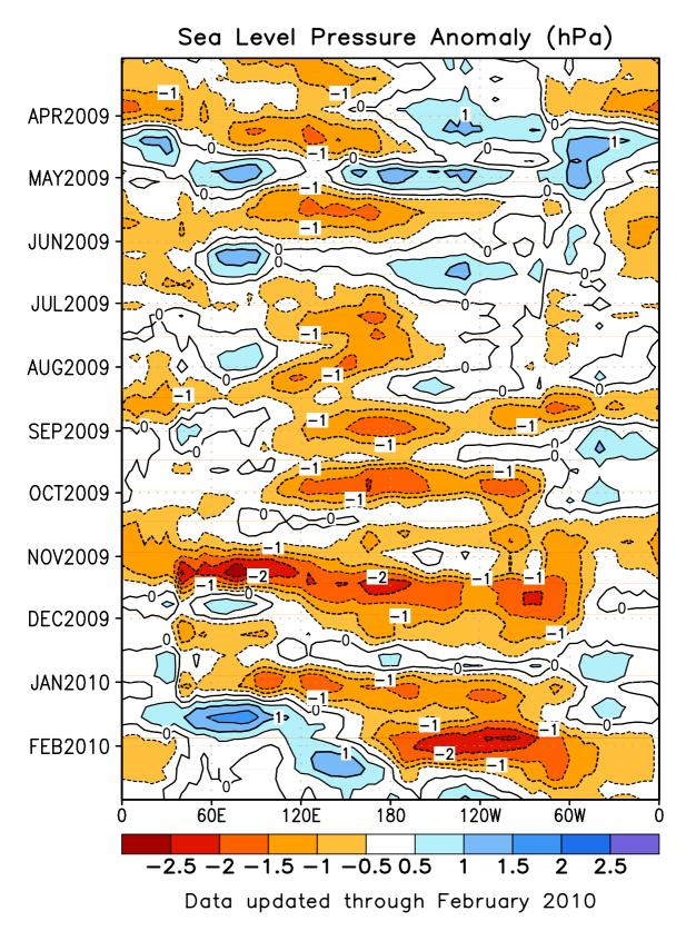
FIGURE T10. Time-longitude section of anomalous sea level pressure (hPa) averaged between 5N-5S (CDAS/Reanaysis). Contour interval is 1 hPa. Dashed contours indicate negative anomalies. Anomalies are departures from the 1979-1995 base period pentad means. The data are smoothed temporally using a 3-point running average.
