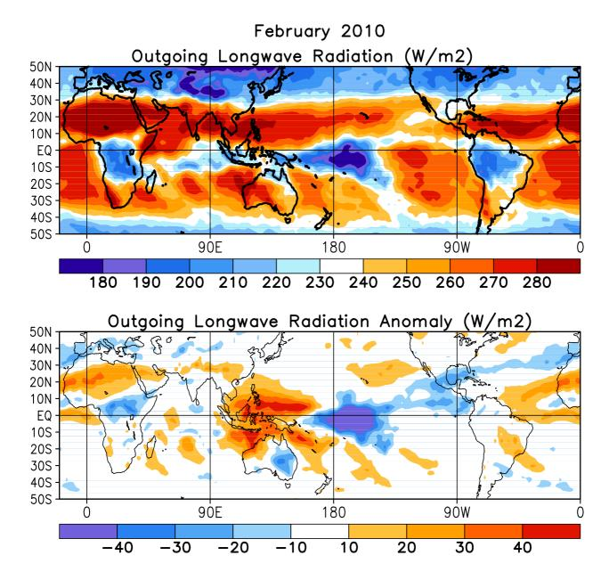
FIGURE T25. Mean (top) and anomalous (bottom) outgoing longwave radiation for FEB 2010 (NOAA 18 AVHRR IR window channel measurements by NESDIS/ORA). OLR contour interval is 20 Wm<sup>-2</sup> with values greater than 280 Wm<sup>-2</sup> indicated by dashed contours. Anomaly contour interval is 15 Wm<sup>-2</sup> with positive values indicated by dashed contours and light shading. Anomalies are departures from the 1979–95 base period monthly means.
