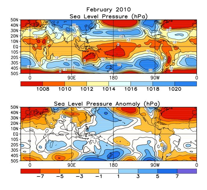
FIGURE T19. Mean (top) and anomalous (bottom) sea level pressure (SLP) (CDAS/Reanalysis). In top panel, 1000 hPa has been subtracted from contour labels, contour interval is 2 hPa, and values below 1000 hPa are indicated by dashed contours. In bottom panel, anomaly contour interval is 1 hPa and negative anomalies are indicated by dashed contours. Anomalies are departures from the 1979-1995 base period monthly means.
