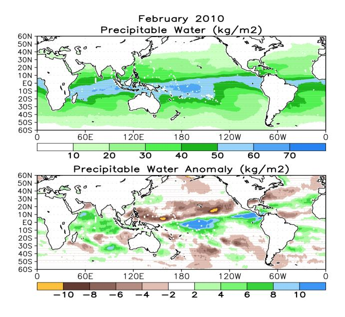
FIGURE T28. Mean (top) and anomalous (bottom) vertically integrated water vapor or precipitable water (kg m<sup>-2</sup>) based on the Special Sensor Microwave/Imager (SSM/I) (Ferraro et. al, 1996: *Bull. Amer. Meteor. Soc.*, **77**, 891-905). Anomalies are calculated from the 1987-2006 base period means.
